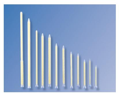
STATOMIX® MS series plastic disposable mixers, when used with meter mix equipment, provide a low cost solution for 2-component mixing. The mixer element is molded of polyacetal to withstand the higher pressures of meter mix machines.
